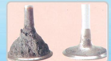
Cars without Cyclone find carbon deposits on intake valves in an efi engine, in addition to other apparent adverse conditions. When carbon accumulates on the intake valve in a fuel-injection system, engine stalling and hesitation occurs, which may lead to valves cracking.
